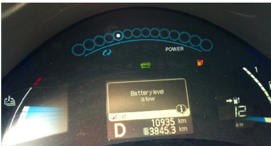
First Stage Low Battery Warning on
